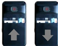
2. Insert the SIM card into the slot. The gold contacts of the SIM card should go against the metal contacts of the phone. Put the contacts of the battery into the hole located at the bottom of the unit insert and press the upper side of the battery until you hear the "click".
