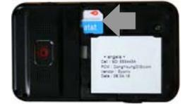
3. To remove the battery push the bottom of the battery to upwards(1) and remove(2) the battery.. Push the SIM card in the arrow direction as shown.
