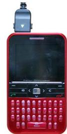
2. To remove the adapter connection press the adapter's side buttons(1) and pulling the adapter away(2).
