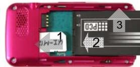
3. To remove the battery push the top of the battery downwards(1) and remove(2) the
