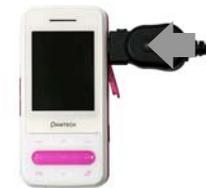
2. To remove the adapter connection press the adapter's side buttons(1) and pulling the adapter away(2).
