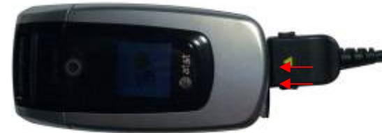
When your battery is fully charged, remove the adapter connection from the outlet, then disconnect the adapter from your phone by pressing the adapter's side buttons and pulling the adapter away from your phone, as shown below.
