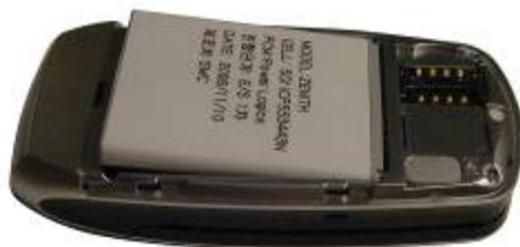
2. If the SIM slot is empty, insert the SIM card into the slot.
