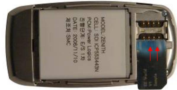
3. To remove your SIM card, push the SIM card in the arrow direction as shown below.
