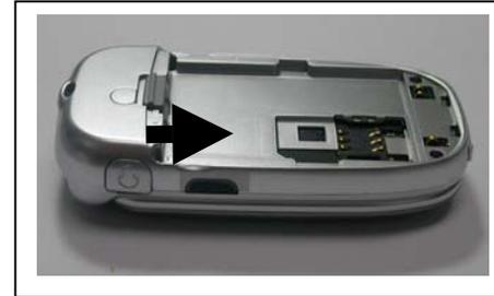
3. If you want to remove the SIM card, push the SIM card in the arrow direction as shown in the picture below.
