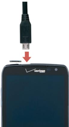
A computer can be also used to charge the smartphone by connecting via the USB cable.
