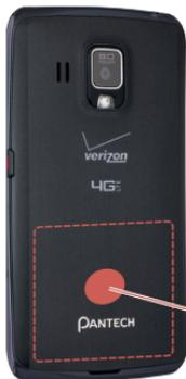
Align this point with an NFC device.
