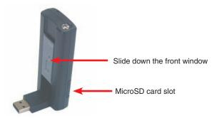
To use this device as Mass storage unit, you must insert optional MicroSD Card in the slot located in the right down side of this device. If there is no microSD in the unit, following alert message will show in the screen.
