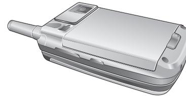
**NOTE:** Make sure the battery is securely placed to avoid slipping off during a call.
