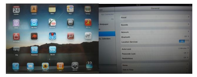
(3), input password and establish a connection, IPAD into search state, looking for bluetooth devices and search to bluetooth keys, search to bluetooth keyboard after hints you on the keyboard input password, right now you need to IPAD on tips according to on the keyboard input corresponding password and press the ok button on a keyboard.
