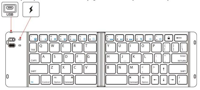
(2). When you charging, the red light on. When the light off, the battery is full enough.(theoretical charging time 2hours)
