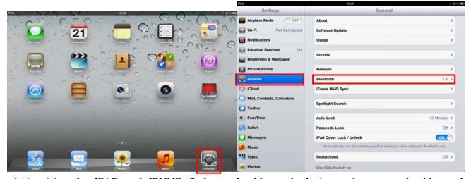
(4). After the IPAD and IPHNE find out the bluetooth device and connect the bluetooth keyboard(see blow picture), IPAD will advise you input the password. Then press "Enter"key.
