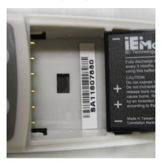
3. Once you slide the battery in it will drop down into base. Press firmly to ensure it is in the base as shown below.
