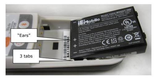
2. Place the battery in the base at an angle to ensure the label side of battery is facing up; make sure the ears on battery line up with the inside of the base (shown below).
