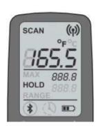
5. The TMD 2.0 searches for a suitable PAR approved RFID tag that has temperature sensing capability.
