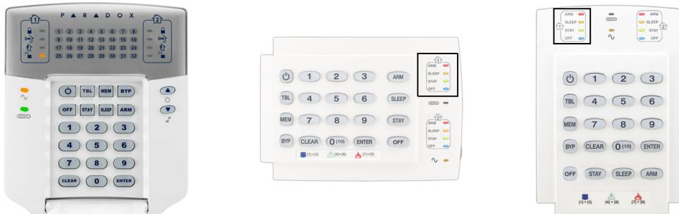
Each time the **[ENTER]** key is pressed, the keypad will display the next digit in the current section and will continue through all the following sections one digit at a time without changing the programmed values. Not available for sections using the Multiple Feature Select Method. Press the **[CLEAR]** key at any time to exit the Data Display Mode.
