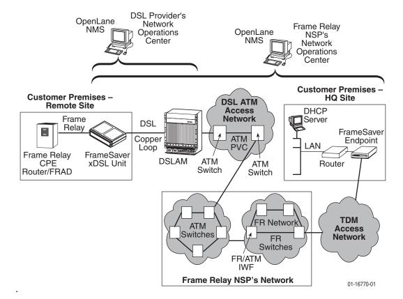
The illustration below shows a typical network configuration that includes a FrameSaver DSL Router.
