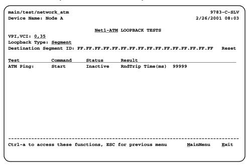
The ATM Loopback causes the FrameSaver device to send either a segment or end-to-end loopback packet toward the network on the selected VCC, then wait for a response.
