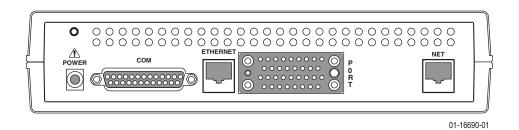
Figure E-2. Model 9783 CSU/DSU Rear Panel
