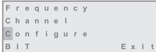
2. Ensure the Configure menu is displayed. Turn the switch until Standby is highlighted, then press the switch.
