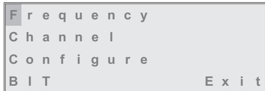
2. Ensure the Set Frequency menu is displayed and that the MHz digits are highlighted. Press the switch.
