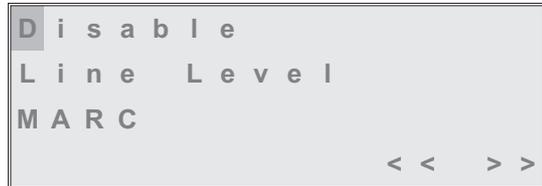
Check that the Disable menu is displayed and Disable is highlighted. Pressing the switch toggles between On and Off. When the correct setting is displayed turn the switch clockwise to highlight OK, then press the switch. You are returned to the Settings menu.
