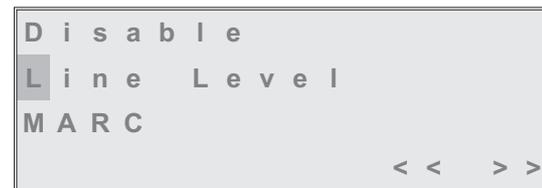
Check that the Line Level menu is displayed and that Line Lvl is highlighted, then press the switch.
