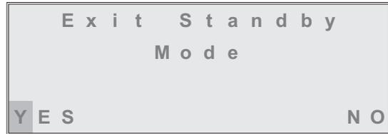
2. Turn the switch until YES is highlighted, then press the switch. [To abandon this procedure, select No instead of Yes and then press the switch.]
