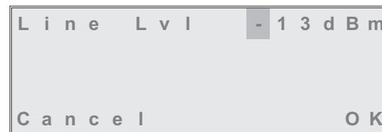
Turn the switch clockwise or anti-clockwise to increase or decrease the value. When the required value is displayed, press the switch. Turn the switch to highlight OK and then press the switch. You are returned to the Settings menu.
