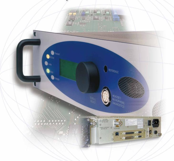
The use of innovative RF engineering allied to sophisticated DSP technology provides class leading performance. The advanced design of the T6TR transceiver allows operation in demanding co-site conditions, reducing the need for external filters. The transmitter employs a sophisticated feedback technique that minimizes spectral noise and enhances signal purity. The power amplifier is designed for optimum performance and maximum reliability and will support continuous operation applications.
