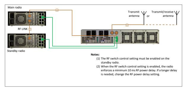
Transmit or transmit/receive antenna with a *Park Air Z4 Solid State Changeover Relay* (which is referred to in this section as a solid state relay):
