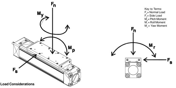
It is important to consider the parameters of the application to best select an actuator. Should the actuator experience difficulties during use, it may be necessary to consider the application when searching for a cause.
