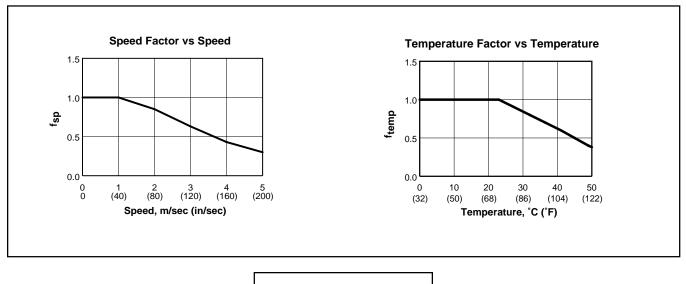
Calculate Effective Load ( $L_{eff}$ ):  $L_{eff} = L_{act} / (f_{sp} \times f_{temp})$
