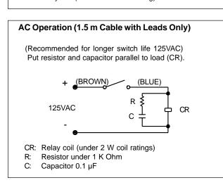
**Note:** Care must be taken not to exceed the Power Rating of the switch while still observing the voltage and current limitations.
