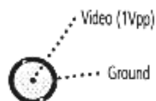
Composite Video BNC Connector (75 ohms)
