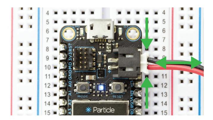
The micro B USB connector on the Xenon is soldered on the PCB with large surface pads as well as couple of through hole anchor points. Despite this reinforcement, it is very easy to rip out the connector if too much stress is put on in the vertical direction.
