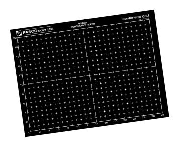
PASCO's PK-9025 Conductive Paper is designed for plotting equipotentials and electric fields. Its resistivity is approximately 5,000 ohms per square. Electrical contact to the paper should be made either with clean, smooth metallic probes, or with the "lead" of a soft graphite pencil. The paper should be used with the PASCO PK-9031B conductive ink pen.
