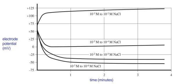
**Figure 4**Typical sodium electrode time response to step changes in NaCl
