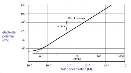
**Figure 3**Typical sodium electrode calibration curve
