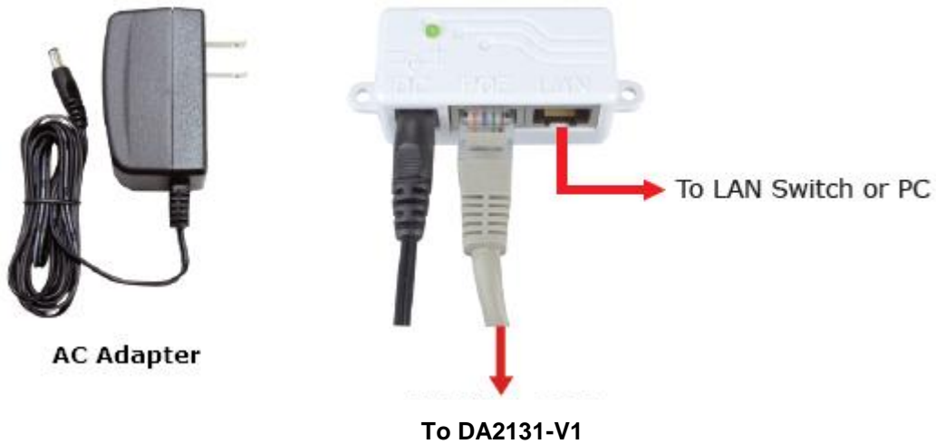
Figure 2-4 Connect to PoE Injector
