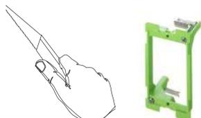
**2** Run a Cat 5 cable from the enclosure location to the single-gang electrical box in the wall at desired Bridge mounting location, and terminate both ends to the TIA/EIA 568A wiring standard with RJ45 plugs.
