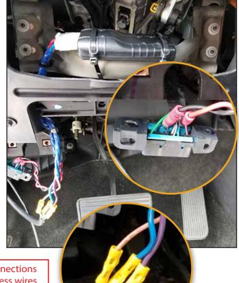
NOTE: When making these connections, use grommets if wires must penetrate the firewall and use adequate looming if placing wires in the engine compartment to protect from hot metal surfaces and corrosive liquids.
