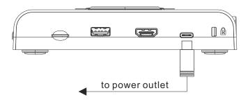
When the battery is full, you can remove the power cord and power it directly through the battery Next ,press and hold the power button for five seconds . Boot-up time is approximately 60 seconds.
