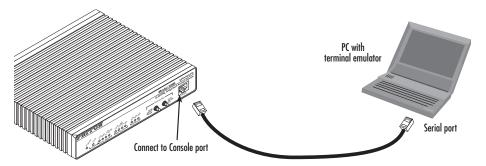
Figure 1. Connecting the ipRocketLink console port to the PC's RS-232 serial port
