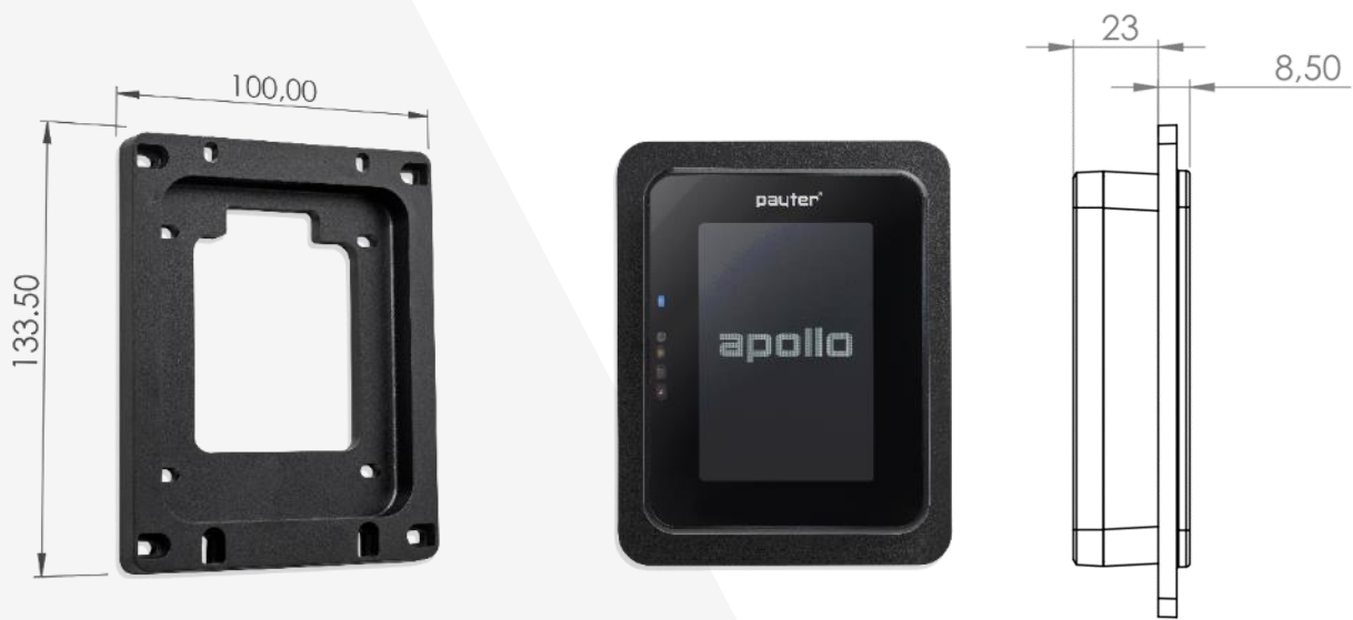
Figure 11: Dimension Apollo terminal without frame
