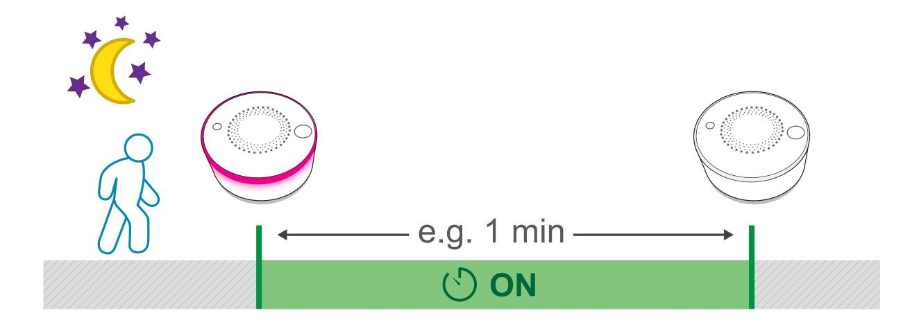
Option 2 works the same as Option 1 but is additionally controlled through motion sensing and a timer as follows:
