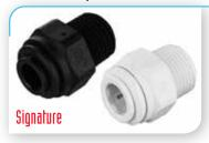
The Ideal H20° John Guest fitting line offers a wide range of push-fit quick connect fittings for pure water applications. These fittings are the world's first food quality push-fit fitting. They provide the quickest and most effective installations with the quality assurance you would expect. Pushing the tube into the fitting is all that is needed to produce an instant but permanent leakproof connection. The fittings are
