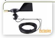
Wind vane uses German Hall effect sensor for precision and durability. Many potentiometer type wind vanes have a dead spot of several degrees, friction from the sensor and a defined life span. Agrowtek's wind vanes have zero dead band, are near-zero friction and have a theoretical infinite life. Includes mounting brackets and 25 ft of outdoor rated cable. Extend
