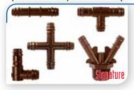
Hydro Flow®/Netafim's 12 mm EZ Dripline fittings are a one-piece construction for added strength, durability and long-term performance. The 12 mm dripline fittings are barbed fittings for a secure fit and easy installation without clamps, glue or tools. Its UV resistance withstands heat, direct sun and harsh chemicals. The 12 mm design fits Techline EZ with inside diameter of 12 mm. Maximum recommended
