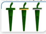
VEW Use the 60° 1/4 inch Long Plunge Drippers with Drip Shields or utilize them as stand-alone drippers. Deliver water and nutrients straight to the root zone of your plants with the subsurface design, which allows the drops to fall 3/4 inch below the surface and dispense out of the three slots at its bottom. 1/4 in barbed nozzle. Self-Cleaning, pressure compensating torturous path. Reusable and
