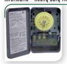
Heavy duty lockable metal enclosure. Tamper proof design. 1/2 in & 3/4 in knock outs. T101 - 120 volt/ SAC/60 Hz/Single pole/Single throw/40 amp. T104 - 208 to 277 volt/AC/60 Hz/Double pole/Single throw/40 amp. 1 Year Warranty.
