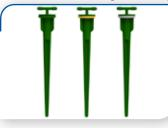
The 6 in Long "T" Rocket Drippers have rocket wings to add to the stability inside of the media. These drippers are great for both indoor and outdoor use. Deliver water and nutrients straight to the root zone of your plants with the subsurface design, which allows the drops to fall 1-1/4 in below the surface and dispense out of the three slots at its bottom. 1/4 in barbed nozzle. Reusable and made from BPA and lead-
