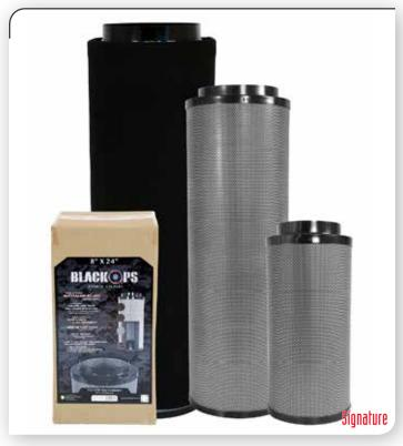
Feature virgin activated Australian RC-4/12 granular carbon that absorbs and traps pollutant molecules within the carbon removing contaminants, odors and impurities from the air. Machine packing allows for more carbon and less movement. These filters are light-weight and have powder coated aluminum tops & bases. They have a built in flange and 2 pre-filters are included. 2 year life expectancy.
