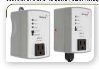
The BPR-1a Basic Power Relay is designed to allow seamless integration of controllers, devices and equipment. The BPR-1a can operate in a Normally Off mode – where the trigger cable activates attached devices – allowing controllers or timers to operate multiple pieces of equipment or larger amounts of amperage. The BPR-1a can also operate in a Normally On mode – where the trigger cable
