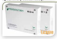
Four, six, eight or 12 dry-contact pilot relays for equipment with GrowControl™ series controllers. Normally open independent contacts allow control of customer relays, contactors and HVAC signals. Removable base-mounted relays for easy maintenance. Terminals rated 120 Volt ac/5 Amps. 2 Year Warranty.
