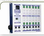
The Powerbox® DPC-24000-BT is our largest and most advanced model so far. This unit has everything you need to run up to 24 1,000 Watt lights, plus accessories at 120V. Best of all, this unit contains our exclusive new 6-channel timer, which allows you to control outlets in six separate zones, making this the most versatile lighting controller available on the market. Main circuit protection is provided by a
