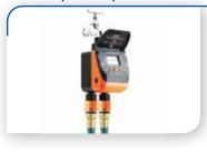
2 independent outlets programmable in advance; watering cycles run on all days of the week. Each outlet releases water up to 3 times a day, for durations ranging from 1 min to 23 hrs and 59 min. 15 min preset manual override allows for watering between cycles or programs interruption. Low-battery indicator; saves settings for 10 min while 9V battery (not included) is replaced. 2 Year Warranty.
