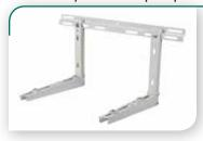
These Wall Brackets are used for supporting condensing units. This wall mount bracket features a cross bar that is attached to a wall and two L-shaped brackets that are hooked and bolted into place on the cross bar. The condensing unit is mounted onto the L-shaped brackets and fastened using the bolts and antivibration washers provided.
