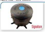
Octa-Bubbler® is a pressure compensating device with a 1/2 inch FPT inlet and 8 swivel port 3/16 inch outlets. Constructed using ABS plastic. Built in back flow prevention engineered for added protection. Octa-Bubblers deliver water to multiple locations. Optional port plugs are available for unused ports. Each Octa-Bubbler® has a 150 mesh filter screen for clog resistance. Interchangeable color coded flow control gives
