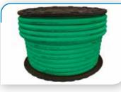
Made in the USA, the ColorStorm™ Premium Rubber Hose is molded from quality EPDM rubber, which will not crack, check or separate. This Premium Rubber Hose resists kinking, coils easily and is flexible to -25° F. It also withstands hot water up to 160° F and has a working pressure of 125 PSI. Crush proof nickel-plated couplings complete this quality hose that is guaranteed for life. Great for creating your own
