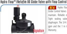
NEW Hydro Flow® by Netafim Series 80 Globe Control Valves are simple to operate and maintain. Reliable even in harsh conditions. Tight sealing valve with fully supported diaphragm. The 3/4 in flow range is 0.01 - 26 gpm and the 1 in is 0.01 - 44 gpm. 1 Year Warranty.
