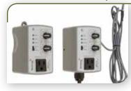
The BTC-1a Basic Temperature Controller is designed to control fans, heaters, air intertek conditioners and other equipment in gardens, greenhouses, grow rooms and other environments. It can operate in either cooling or heating modes. The BTC-1a features a readily visible switch to alternate between cooling and heating. Easyto-read dials make programming daytime and nighttime settings uncomplicated. 2 Year Warranty.
