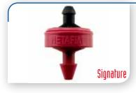
Hydro Flow® by Netafim Woodpecker Pressure compensating junior dripper with built in check valve and barbed outlet. These drippers adjust themselves automatically to the system pressure resulting in a watering uniformity, even on slopes. Since all water is delivered directly to the container, there is no run-off, saving water, fertilizer and energy. These drippers can be used in conjunction with dripper stakes and spray
