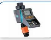
Programmable in advance to release water up to 2 times a day, for duration ranging from 1 min to 23 hrs and 59 min. Weekly programming; water cycles run on all days of week. 15 min preset manual override allows for watering between cycles or programs interruption. Lowbattery indicator; saves settings for 10 min while 9V battery (not included) is replaced. 2 Year
