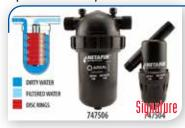
Disc Filter technology has grooves in the disc rings that criss-cross to form a network that traps debris between and on the outside of the discs. As dirty water is pumped into the filter and pressure increases, the water compresses the disc rings together tightly. The water is then forced to flow through the grooves of the disc rings, where debris is trapped, releasing only clean water to the irrigation system.
