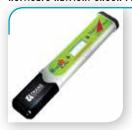
Trans Instruments HortiCare Nutrient concentration check tester is specially designed with advanced features to ensure fast and accurate concentration test, for the commercial as well as home growers. Operating Range: 0 to 1,990ppm; Display Resolution: 10ppm; Accuracy: ±5% full scale; Calibration Point: 990ppm (KCI); Battery: 4 x 1.5V Button Cell (LR44 equiv.).
