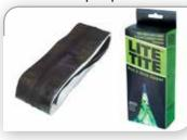
Black Tear Proof Tape Designed for use with ordinary construction vapor barrier. This adhesive-backed zipper is perfect for creating a simple, resealable access doorway. The 84 in long, heavy-duty, water proof #5 zipper is sewn to a 950-denier high-density polyethylene backing that has a permanent high-tack acrylic adhesive.
