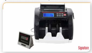
The High Roller® LCD Bill Counter features both UV (ultraviolet) and MG (magnetic) automatic detection while counting. Automatic start, stop and clearing functions. It has a front LCD display, side display and includes an external plug in display. Counting speeds of up to 1000 bills/min. Highly accurate counting of bill quantity. Does not count denominations.
