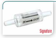
EcoPlus® Check Valve is a must have for every air pump. This product helps prevent back siphoning of water which can damage pumps or even flood water into your rooms. This check valve works by allowing air to flow in one direction and blocking water from getting too far down your air tube. Simply connect the Check Valve between the air pump and airstone. Works with 3/16 in ID air tubing.
