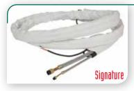
NEW ReFlex™ line sets are used to simplify installation of HVAC split system equipment. By connecting the indoor evaporator along with the outdoor condensing unit, this system allows an easy installation with out the headache of kinking copper tubing and saves on install time and labor. The ReFlex™ line set comes pre-wired, pre-insulated and also comes with flare fitting on both ends, with an
