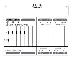
Front view of a C-Bus Changeover Relay
