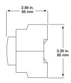
Side view of Network Bridge showing height and depth
