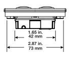
Top view of keypad showing width
