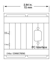
Front view of the PC Interface showing width
