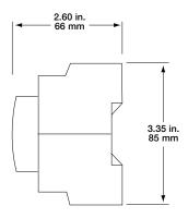
Side view of a C-Bus Changeover Relay
