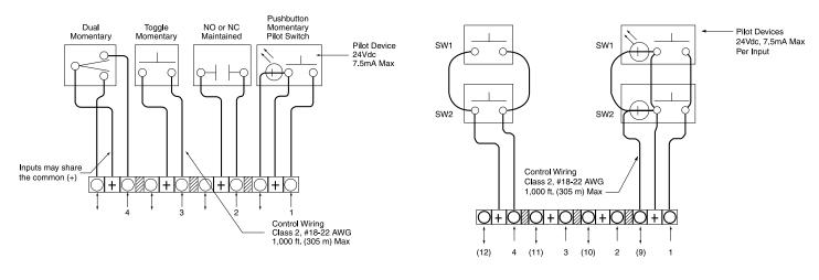
Typical Switch Types Wired in Parallel
