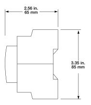
Side view of a C-Bus 4 Channel 10 Amp Relay
