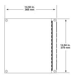
Front view of 24M Enclosure box showing height and width
