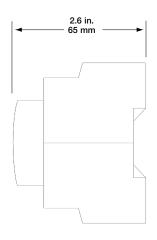
Side view of Four-Channel Auxiliary Input Unit
