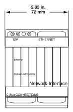
View of the Ethernet Network Interface showing width
