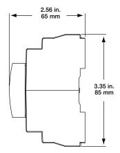
View of the Ethernet Network Interface showing height and depth
