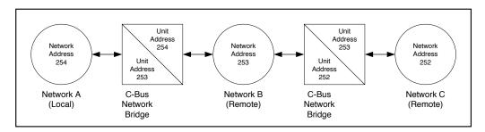
Multiple C-Bus networks connected in series using C-Bus Network Bridges
