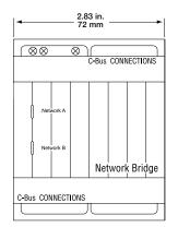
Front view of the Network Bridge showing width
