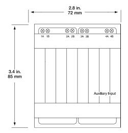
Top view of Four-Channel Auxiliary Input Unit
