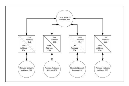
Multiple remote C-Bus networks connected to local network using star topology.
