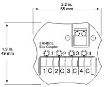
Top view of Four-Channel Bus Coupler
