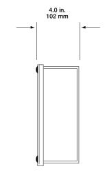
Side view of 12M Enclosure box showing depth
