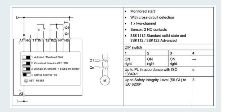
Typical circuit 9: Two-channel, with cross-circuit detection, with autostart
