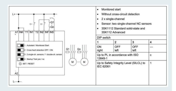
Typical circuit 13: 2x single-channel, without cross-circuit detection, with autostart
