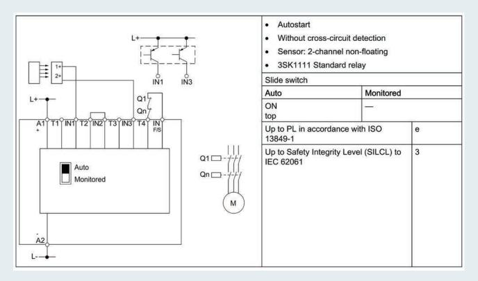
Typical circuits for 3SK1 Standard solid-state basic units or 3SK1 Advanced basic units
