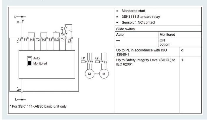
Typical circuit 2: Single-channel, with monitored start
