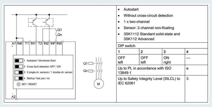
Note: Single-channel connection - If only one single-channel sensor is used, the other sensor circuit must be jumper
