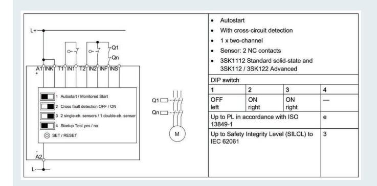
Typical circuit 10: Electronic sensor, 2-channel, without cross-circuit detection, with monitored start
