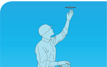
Contact Juno Lighting Group Technical Services for the appropriate replacement and "group re-lamp" all fixtures on the same circuit with new LEDs
