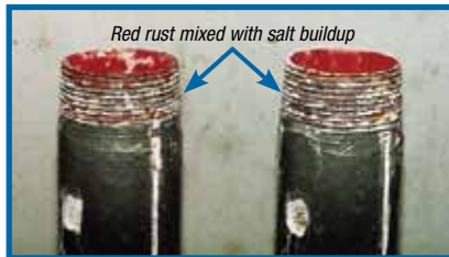
Examples of Spray-Galvanized (Hot-Galvanized) Threads after 42-day salt-fog test
