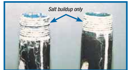
Examples of Hot-Dip Galvanized Threads after 42-day salt-fog test
