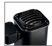
External Linear Grate Provides cutoff and glare control and protects lens from falling objects. Easily attaches to top cover of fixture with four black stainless steel screws (included). Not for use with E-GAGS.
