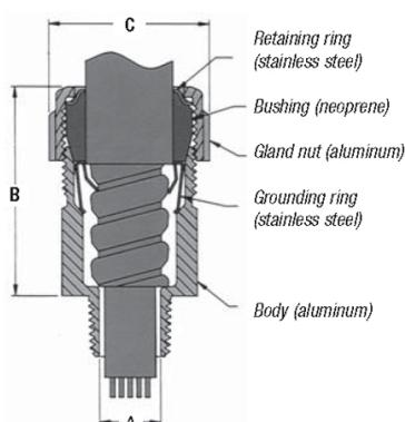
Easy Installation-Exclusive power-grip. Provides a grip that's high up on the cable-not on the first convolution-so strip length and cutting of cable are not critical.
