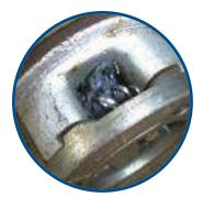
The die teeth are cutting tapered threads and will become clogged with PVC and metal shavings.
