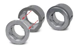
The two-piece 13158 adapter enables the use of SUPER CUT die heads with the MINI-COLLINS™. For dies up to 1-1/4 in. in size, use both pieces together, as shown at right. For larger dies, separate the two pieces, as shown at left, and use only the outer ring.
