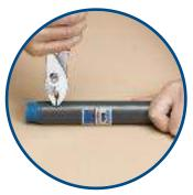
In Step 3, the tab is pulled perpendicular to the conduit with a pair of pliers. The plastic tab will tear off rather than having any peeling effect or the coating separating from the substrate.
