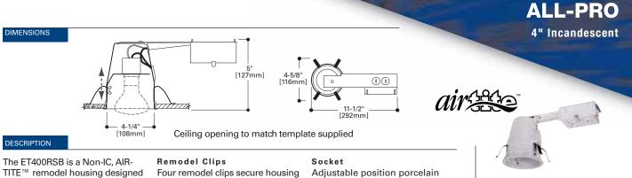
TITE<sup>™</sup> remodel housing designed for use with small aperture trims. The shallow height allows it to be used in spaces where vertical height is limited. The ET400RSB is installed from below the ceiling. For use in non-insulated ceilings.
