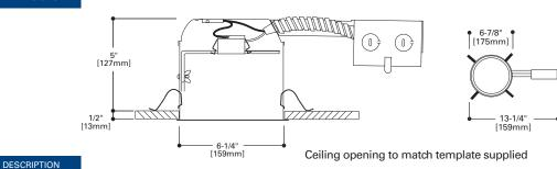
Four remodel clips secure housing
