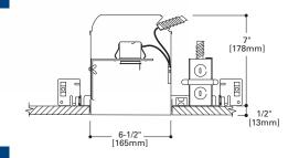
The EI700AT housing is designed for use in insulated ceilings where the housing will be in direct contact with insulation material. AIR-TITE design meets restricted airflow requirements.
