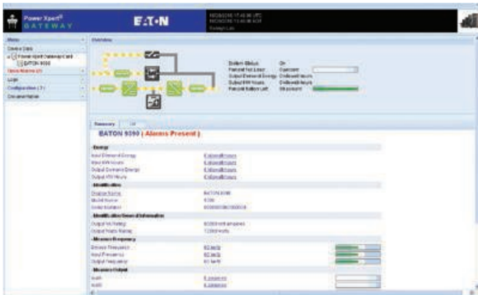
Power Xpert Gateway UPS card homepage
