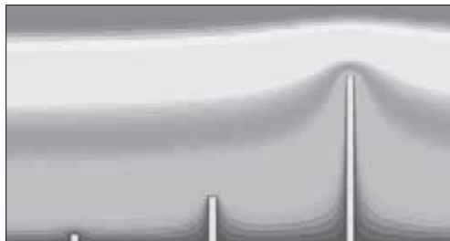
Figure 3. Field intensification, portrayed with lines of equal voltage (equipotential lines), is a function of the height of the object as well as its degree of "sharpness".
