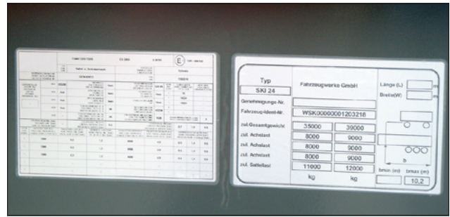
Type plate of an HGV trailer with protective laminate.
