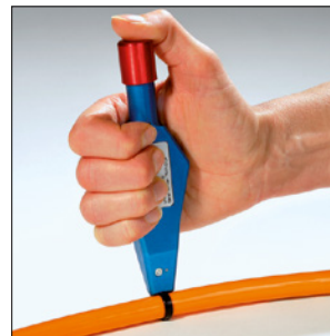
... press on the button whilst maintaining pressure on the tool...
