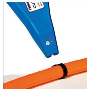
Bring the tool perpendicular to the tie...
