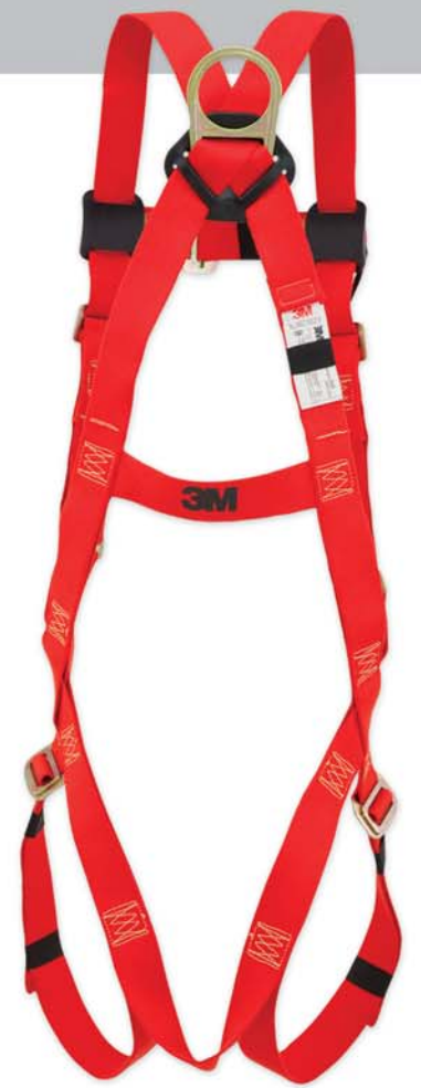
1020 Saturn Welding Harness with pass thru chest connection, pass thru leg connection, back D-ring, 310 lb. capacity (Universal) and 400 lb. capacity (XXL). Universal size and available in XXL
