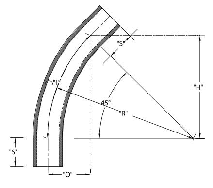
**ETL LISTED CONFORMS TO UL651** ETL CONTROL #3107144 **CONFORMS TO NEMA TC3** SEE NEC ARTICLE 352 FOR USE MATERIAL IS RIGID PVC BEND TOLERANCE IS ±2°
