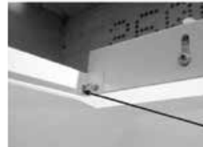
4. Install end spacer bars and tighten screws. Make sure all four corners are squared before tightening. Note: Line up rectangular cut-out slot to the head of the screw and slide in when placing.
