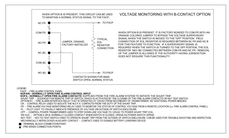
Figure 8. Voltage Monitoring with B-Contact Option.
