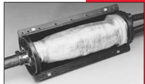
The closure kit provides moisture protection and prevents water migration into the splice bundle. The closure is impact-tough and provides double protection as static air pressure surrounds the encapsulated splice. The closure is reenterable and made for use with (PIC) filled, waterproof cable.
