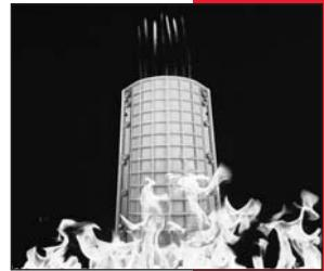
The system has an oxygen index of 28% minimum and a UL 94 rating exceeding V.O. The closure self extinguishes when the fuel source is removed.
