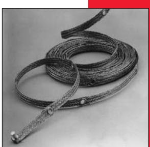
Provides low electrical resistance connections, contributes to strain relief across cables. Eyelets fit shield connector studs up to 6 mm (1/4") diameter. Size: 13 mm x 7.6 m (1/2" x 25'), eyelets spaced 76 mm (3") Size: 13 mm x 7.6 m (1/2" x 25'), eyelets spaced 152 mm (6")
