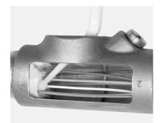
With one of the packing tools, packing fiber in between and around electrical conductors is effortless.
