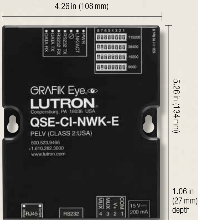
Shown above: RS232/Ethernet interface (QSE-CI-NWK-E)
