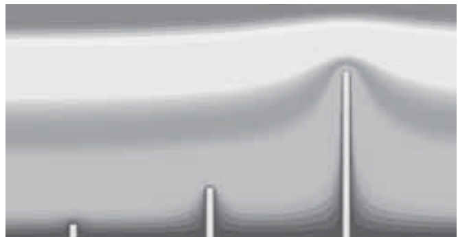
Figure 2. Field intensification, portrayed with lines of equal voltage (equipotential lines), is a function of the height of the object as well as its degree of "sharpness".
