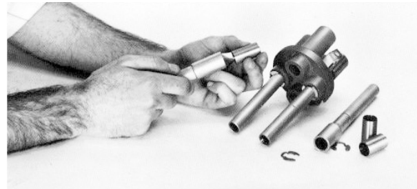
Figure 6. Wire Well Reducer Installation
