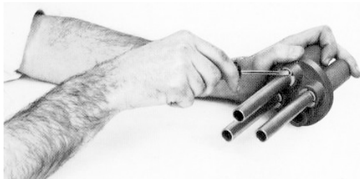
Figure 3. Retaining Clip Removal
