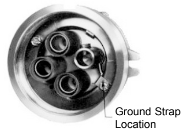
Figure 9. Grounding Strap Location
