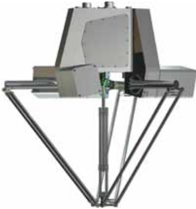
PacDrive Delta 3 robot type P4
