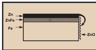
Protection of cut edges with zinc coatings.
